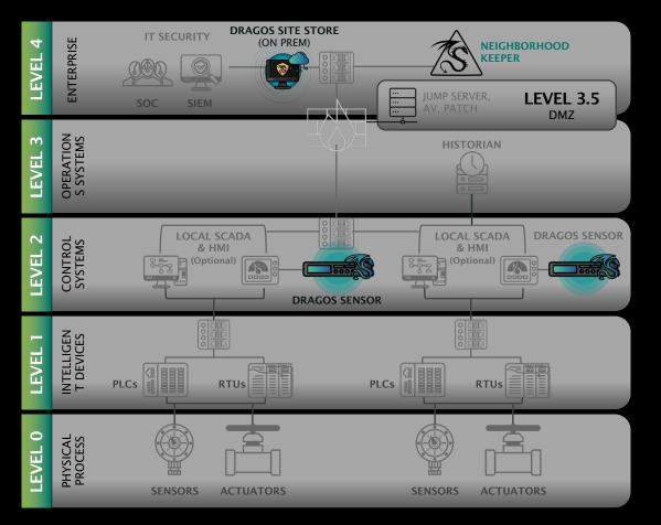
The Dragos Platform's sensor is deployed passively in the ICS/OT Networks such as plant or substation networks.
