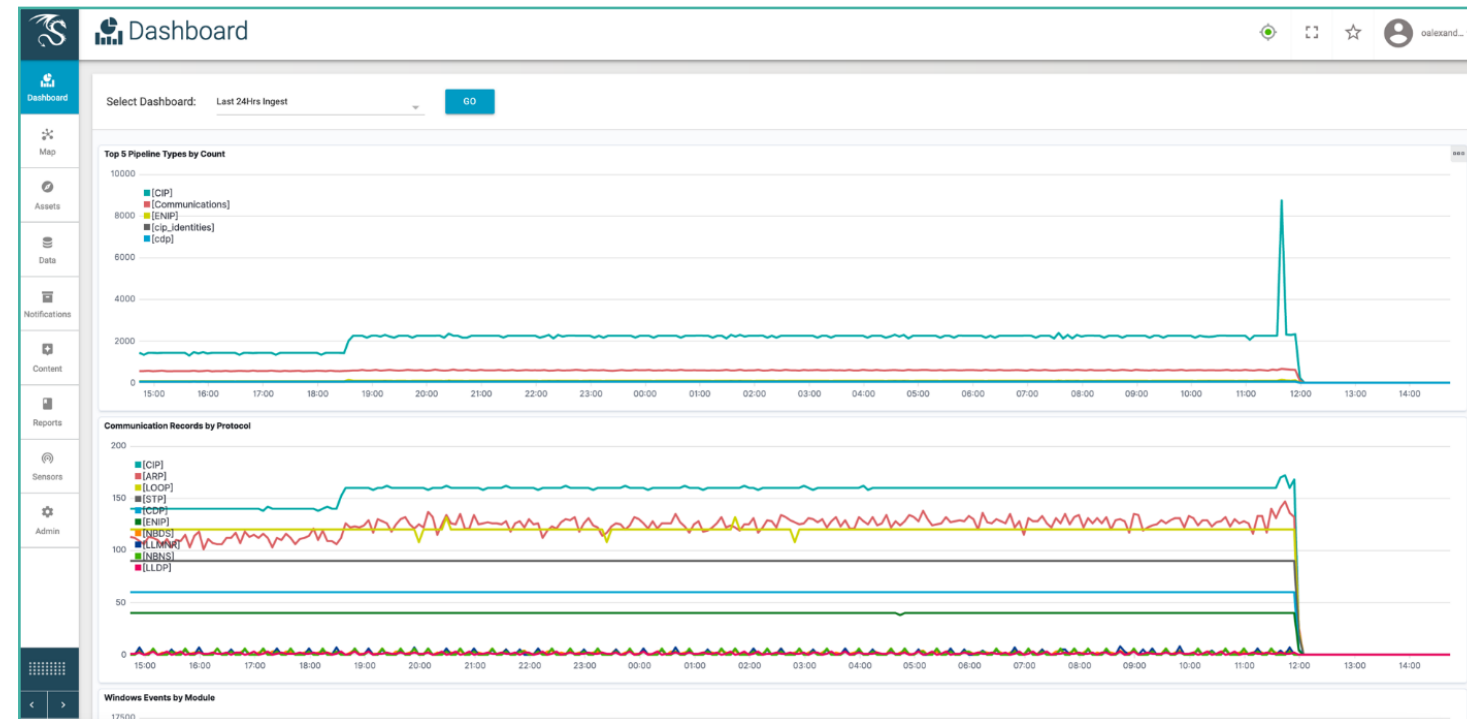
Figure 34: Dragos Platform telemetry of the final Events prior to the plant having a complete communications blackout which we assumed was due to the destruction of the BMS
