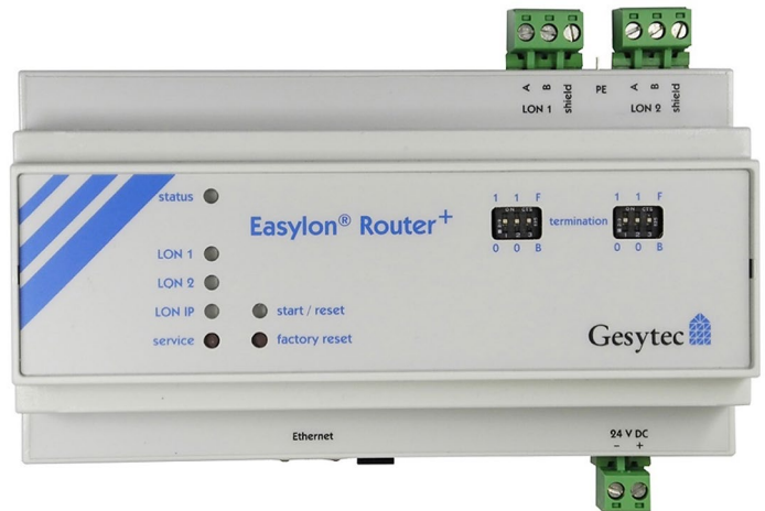
Figure 27. 3-LIP : Level 3 FPOC Router Between Three LonTalk Networks: Level 1 Lon over TP/FT-10, Level 1 Lon over TP/FT-10, and Level 4 Lon over IP over Ethernet
