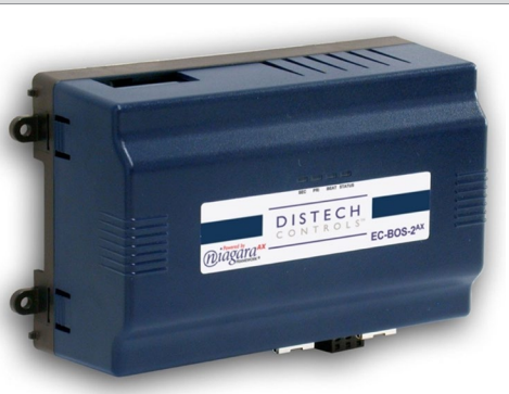
Figure 29. 2A-JACE: Programmable Level 2A controller. No analog inputs or outputs. The primary networking is proprietary over IP over 10/100Mbps Ethernet. For a small field control system, this might be the Level 3 FPOC.
