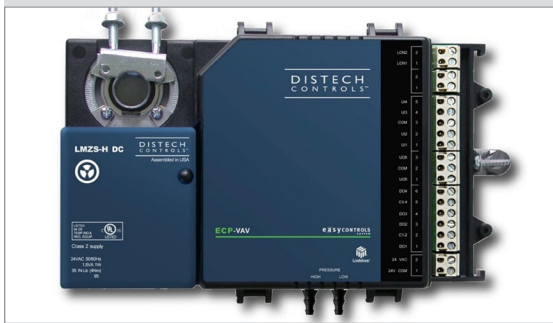
Figure 31. 1A-VAV: Variable air volume (VAV) box controller with multiple analog inputs and outputs. Also incorporates dedicated actuator and pressure sensor (normally Level 0 devices). The network is LonTalk over TP/FT-10 media at 78Kbps.
