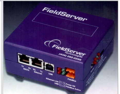
Figure 30. 2C-FS: A Level 2C gateway (application layer proxy). The Level 2 network is Modbus over IP over 10/100Mbps Ethernet. The Level 1 network is proprietary over proprietary 2-wire media.
