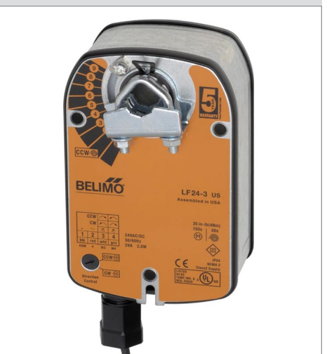
Figure 36. 0-Actuator: Electric motor taking 4-20 mA or 0-10 VDC analog input signal and producing a 90-degree rotation.
